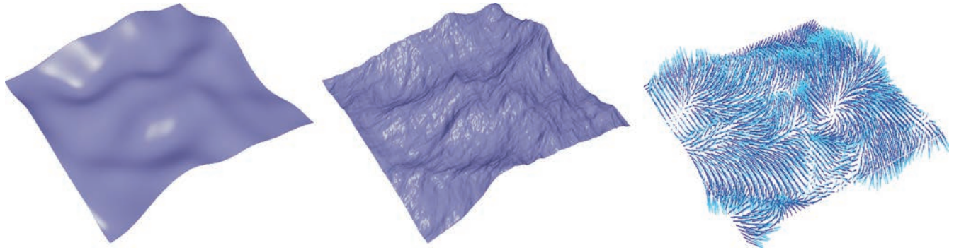
Fig. 1. (Left) Input previs of waves from a visual effects production environment. Only geometry is provided. Angular frequencies and amplitudes vary in time. (Middle) Output synthesized waves. Horizontal displacements and high frequencies have been added based on an estimation of wave parameters (amplitude, phase shift, and angular frequency) for each wave vector present in the input. This enhances the previs with flat troughs and sharp peaks that characterize true deep water waves while retaining a correspondence to and the timing of the previs. (Right) Analytical surface velocities projected onto a plane.
