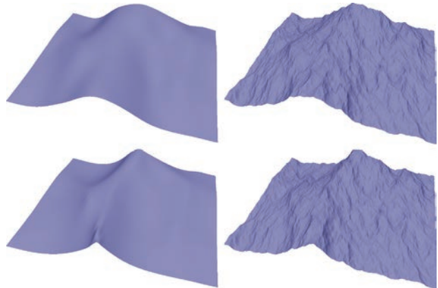
Fig. 6. (Left) Input waves formed by a summation of low-frequency waves based on the Phillips spectrum [Tessendorf 1999]. (Right) Output synthesized waves with horizontal displacements and high-frequency details added. Horizontal displacements have been added to the input surface in the bottom row, but not the top row. Notice how the output surface preserves the sharpness present in the input surface shown in the bottom row.
